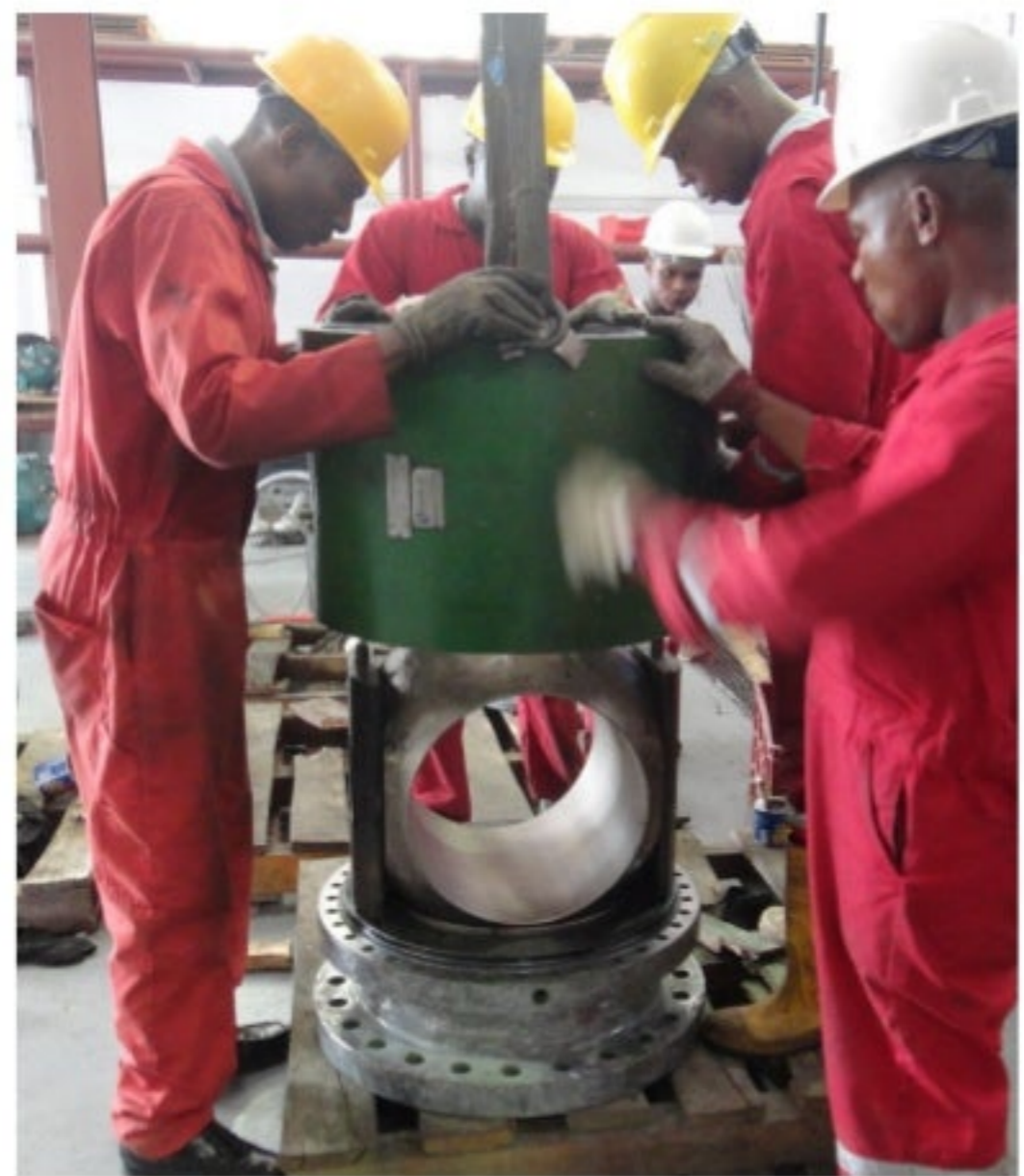
Reassembly of a Ball Valve during corrective maintenance
