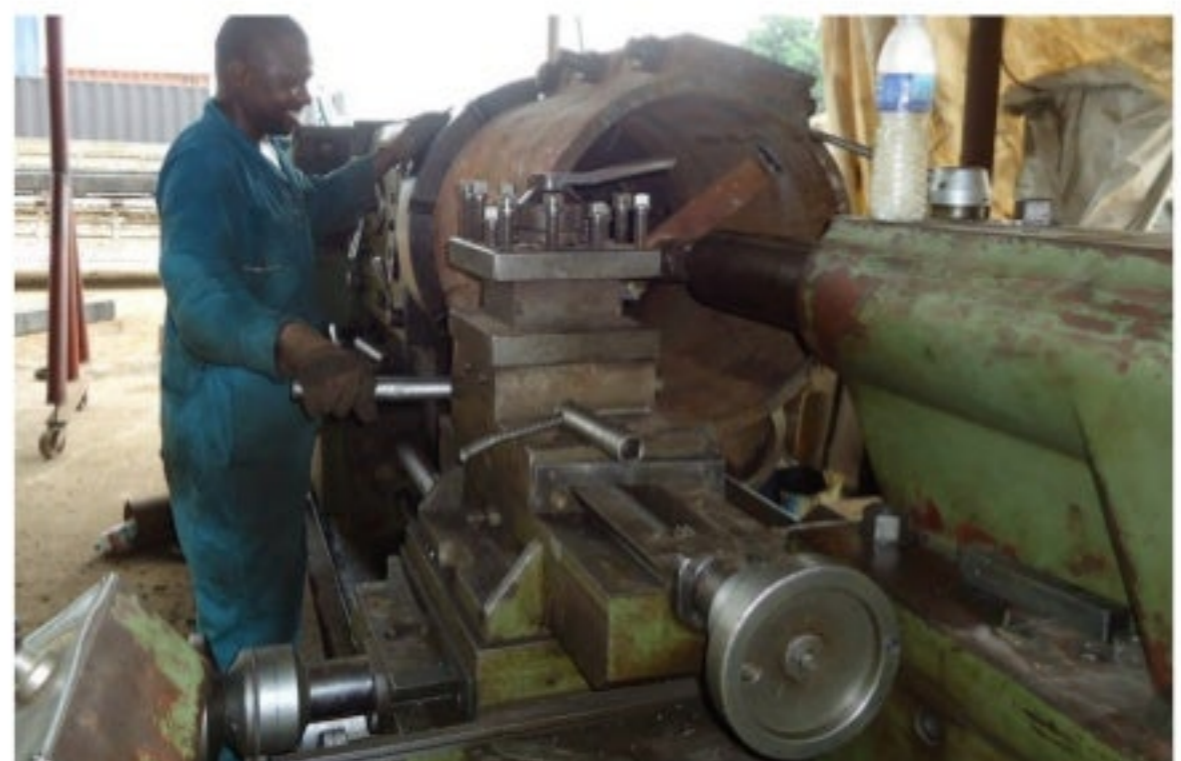
► Valve machining process using a Lathe Machine
